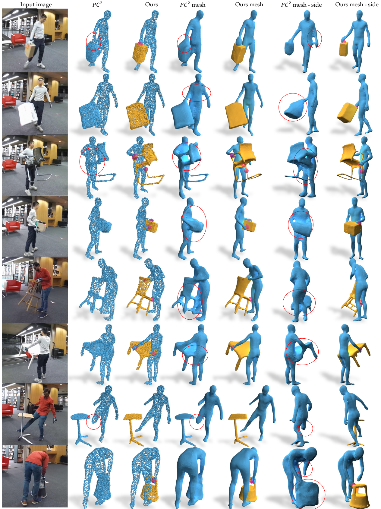
Figure 11. Comparing the shape fidelity of our method with PC 2 on the BEHAVE [7] dataset. PC 2 does not separate human and object and its prediction is noisy, leading to inaccurate meshes. Our method predicts clean point clouds with human object segmentations, allowing us to extract high-quality mesh surfaces.
