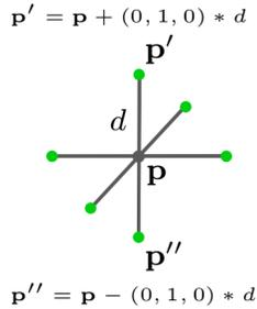
Figure 1. Illustration of locations for feature extraction. In order to add information on the local neighborhood into the point encoding, we extract features not only at a query point’s location  $\mathbf{p}$  itself, but *also* at surrounding points (●) in a distance  $d$  along the Cartesian axes.
