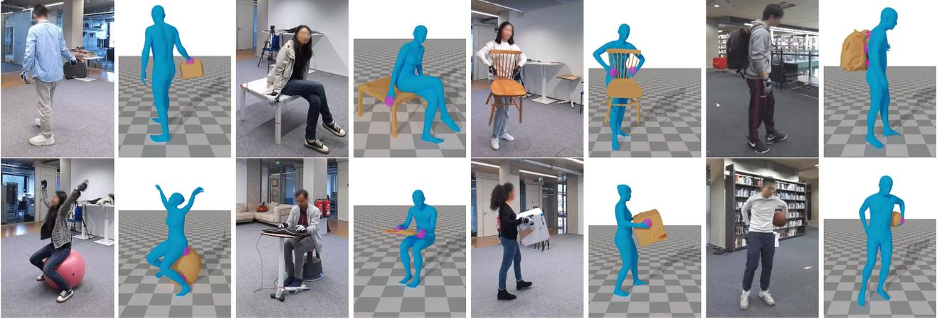
Figure 2. We present BEHAVE dataset, the *largest* dataset of human-object interactions in natural environments. BEHAVE contains multi-view RGBD sequences and corresponding 3D object and SMPL fits along with 3D contacts.
